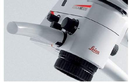
Handles can be removed and sterilized
