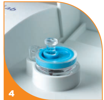
4 Close analyser lid. Result displayed within 4 minutes.
