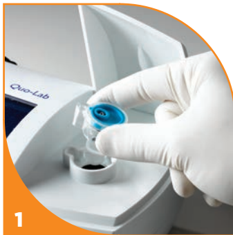
1 Scan lot calibration barcode. Remove foil from cartridge and insert into analyser.
